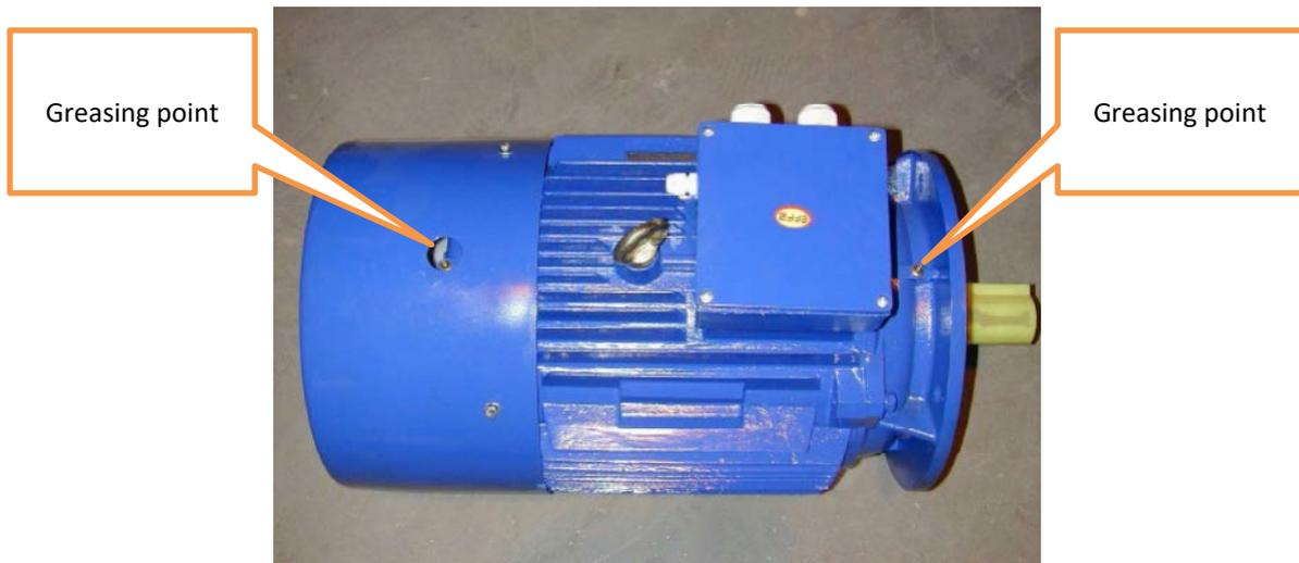
Figure 7-1 – Greasing point electric motors
